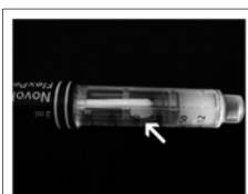
Figure 1. Flexpen used by the patient during the period of metabolic control impairment. Arrow points to the disengaged barb at the tip of the piston rotor.
